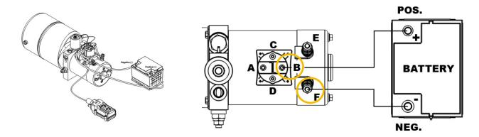
Connect the positive side of the battery to the positive side of the solenoid starter (B), mounted on the electrical motor. Then, connect the negative side of the battery to the ground terminal (F) on the motor.
