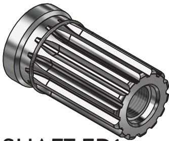
SHAFT FD1 Splined 14-DP12/24 Flat root side fit to fit ANSI B92.1 1996 IMPERIAL
